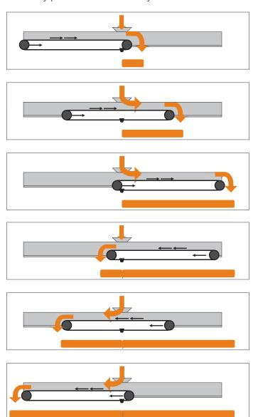
The non-powered belt runs at low tension, meaning long life and easy maintenance.
