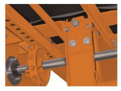
The rack-and-pinion drive for the trolley is simple and dependable. The drive sprocket teeth engage the carriage track for positive no-slip power. The drive is protected by a slip clutch.
