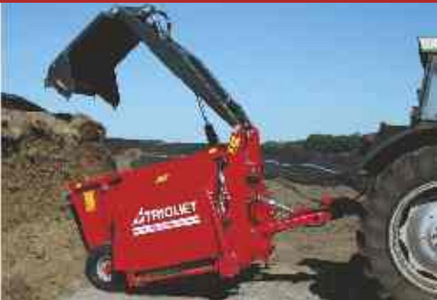
Self-loading feeder-distributor wagon with cutting system Capacity 3 m 3
