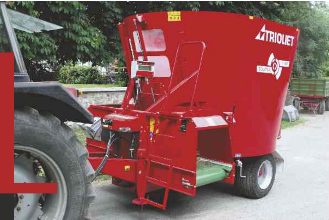
Cross conveyor belt at the back of the machine as an option.
