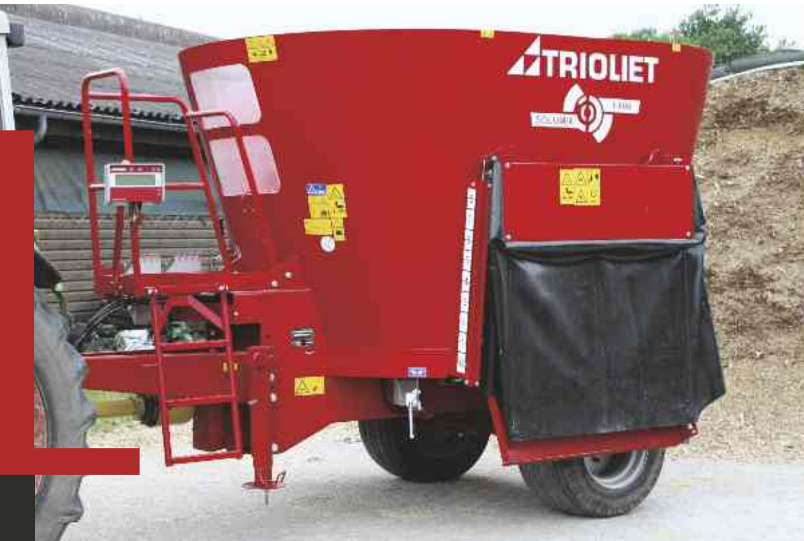
Complete regular discharge by new type of discharge door and door covers.
