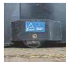
Special rollers underneath the loading platform prevent unnecessary wear to the platform.
