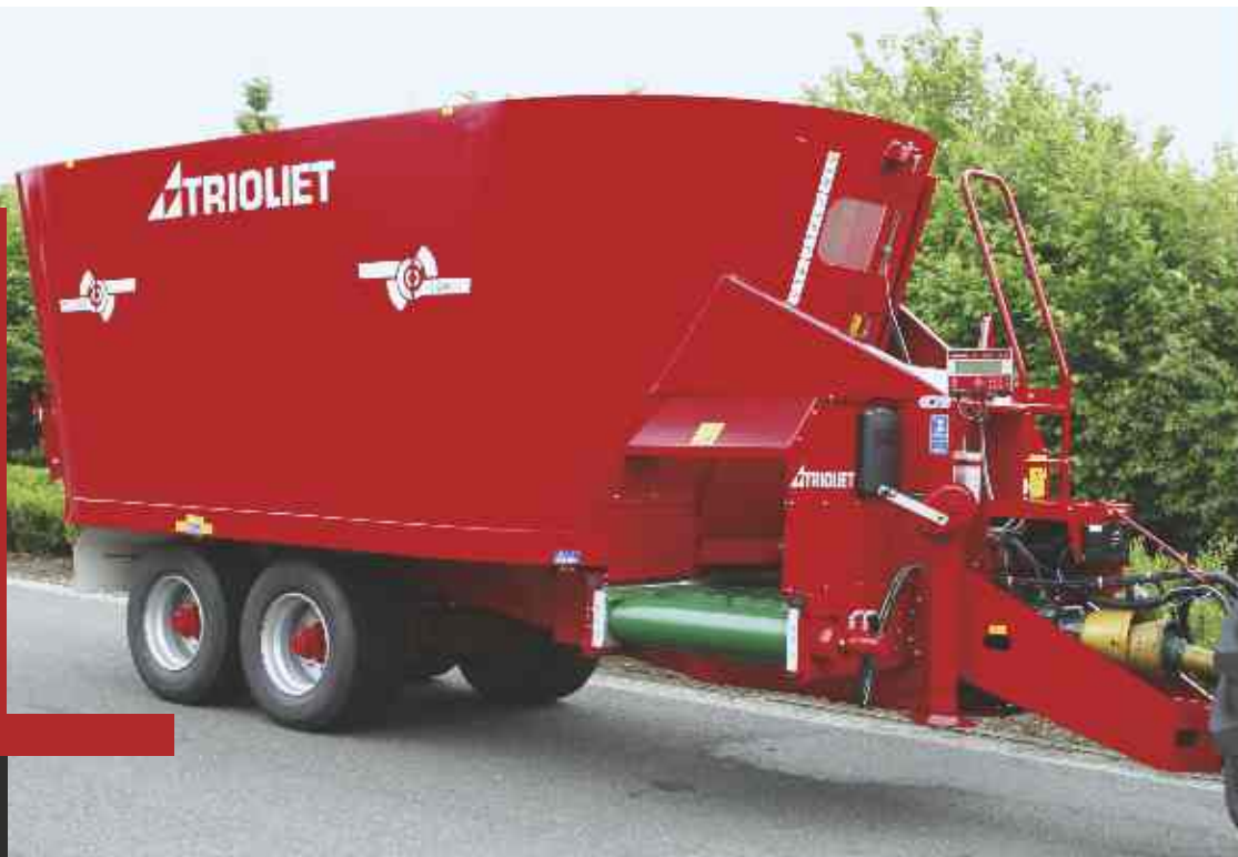
Model VLX-K-T with adjustable chain conveyor at front.
