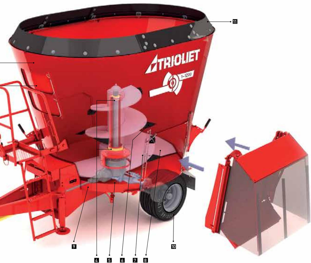
**6 Trioform auger knives: less resistance, less fuel** | The patented shape of the auger knives reduces the resistance. Because of this, fuel is saved. The Trioform auger knives are also self-sharpening and the special shape lead up to a higher strength and long life.
