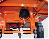
A powerful mechanical brake mounted on the rotor shaft.
